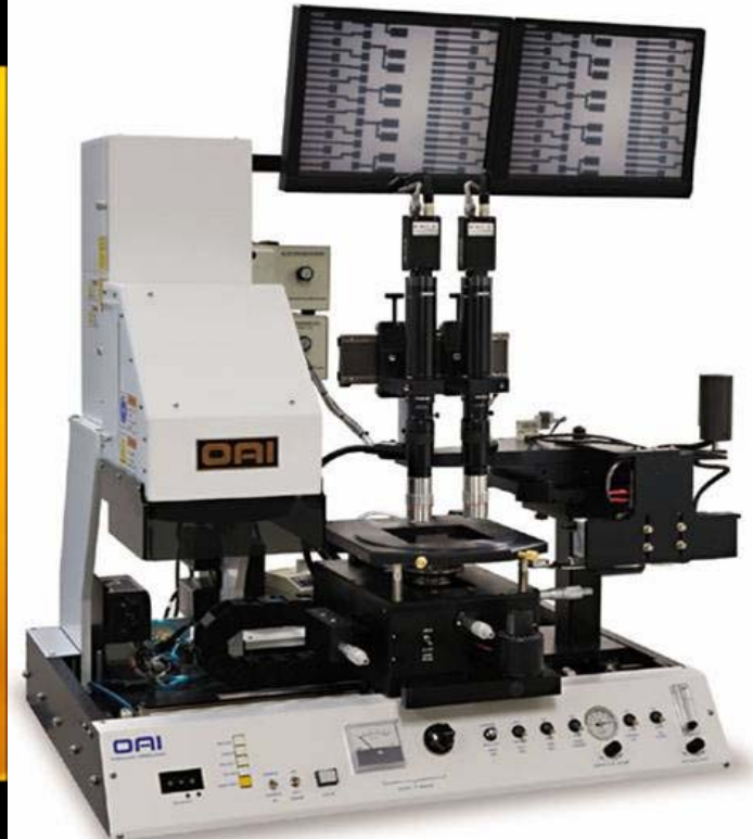
Expose UV through mask
