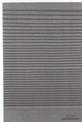
Figure 3. TEM image of Pt/C multilayer
