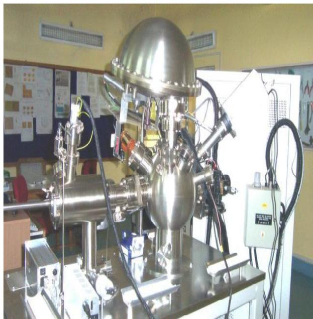
distinguish different chemical environments of atoms; these appear in XPS spectra as core level binding energy shifts. The origin of chemical shifts arises from enhanced or reduced electronic screening of electrons due to charge transfer. Small mean free paths of the photo-ejected electrons make XPS very surface sensitive ( $\sim 1$  nm). The technique of XPS is very useful in the studies of thin film structures, heterostructures, bulk samples, and even for the studies of biological samples.
