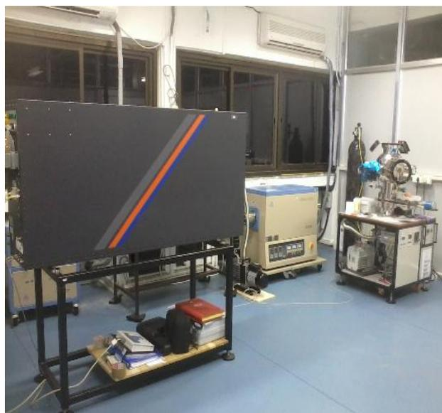
This is a newly installed facility. PLD system helps growing epitaxial thin films of various materials albeit the most preferred materials are oxides. The newly installed system was developed in a piece-wise manner by procuring several modules from different sources. We are depositing epitaxial bi- and multi-layer thin films of superconducting (viz. YBCO) and colossal magneto-resistance (viz. LSMO) on suitable substrates.
