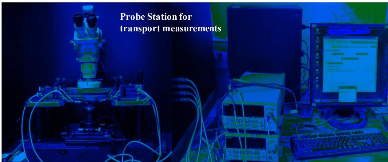
*A Keithley-make probe station is used to study electrical transport properties of nanostructured thin films and individual nano structures.*
