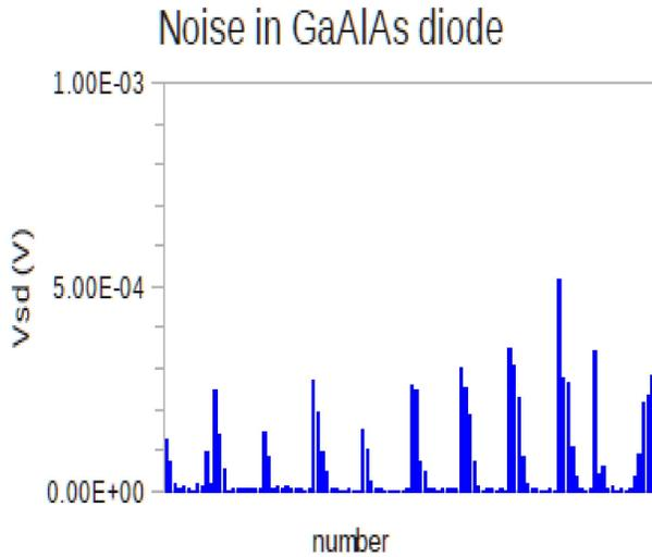
Figure-1:  $V_{sd}$  as a function of number of observations in GaAlAs diode
