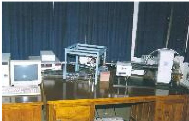
(250-850 nm) detector is available at Cluster & Nanostructure Laboratory. Temperature (down to liquid-nitrogen temperature) effect on luminescence can be studied for semiconductors, oxides and organic compounds. This instrument can identify trap states, band edges of semiconductors and also new organic compounds based on luminescence properties of materials.
