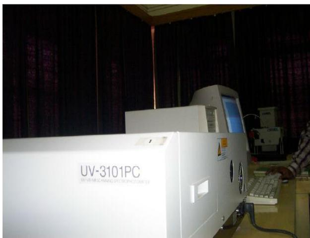
Shimadzu-make UV-3101PC spectrophotometer with PbS detector (for longer wavelengths) is available at Cluster & Nanostructure Lab. The spectrophotometer uses two sets of gratings to cover a wide range of wavelengths (200-3200 nm). Both solid and liquid samples can be used for experiments. Optical properties viz. band gap estimation, quality of the crystal etc. can be studied. The instrument can operate in absorbance, transmission and diffused reflectance mode.
