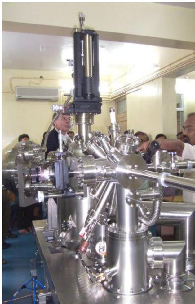
photo excitation. The analysis chamber is also equipped with a 4-axis sample manipulator-cum cryostat, which can go down to 20K. Facility for performing Low Energy Electron Diffraction (LEED) is also available in the analysis chamber. The sample preparation chamber has facilities for scrap cleaning and evaporating metal films.
