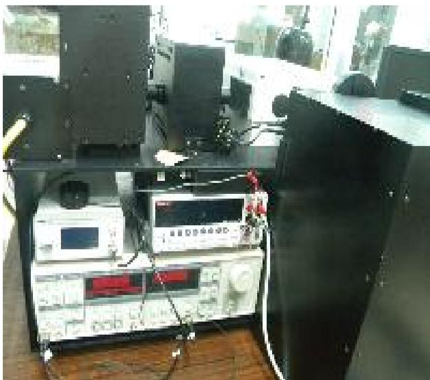
both fed into the precision lock-in amplifier to allow measurement of the photocurrent generated by the modulated monochromatic light.
