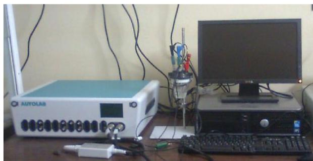
scanned. In cyclic Voltametry experiment the working electrode potential is ramped linearly versus time. The voltagrams are utilized to study the electrochemical properties of an analyte solution. Application areas include conductive coatings, polymers, semiconductors, batteries, fuel cell, super capacitors etc.
