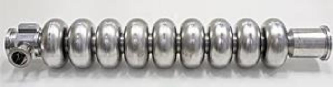
Super conducting acceleration cavity (Homemade by KEK)
