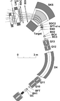
Fig. 1. Schematic view of the E10 beam line spectrometer (from CC to BUC2), the target area (SSD and target) and the SKS spectrometer (from SFT to LC). See the text for more details.
