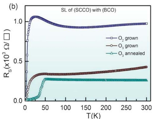
**Figure:** Temperature-dependent sheet resistance for SCCO/BCO superlattices under various condition.
