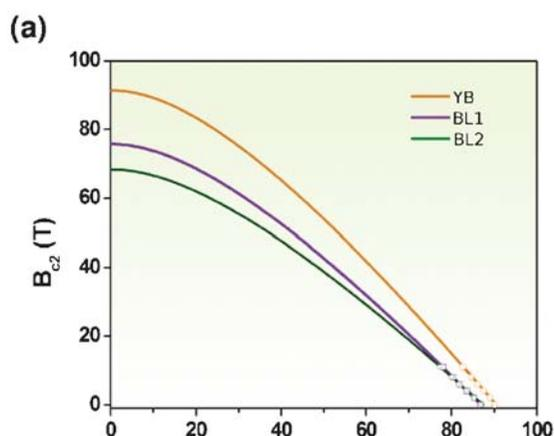
**Figure:** Schematic of the superconducting (YBCO)/ferromagnetic (LSMO) bilayer layer YBCO, bilayer BL1 and bilayer BL2 respectively.  $B$ - $T$  phase diagrams for YBCO (YB) and bilayers (BL1, BL2) constructed from magneto-transport data using WHH formalism with varying LSMO thickness grown on  $\text{LaAlO}_3$  (LAO).  $x = 0, 16$  and 28 for single.
