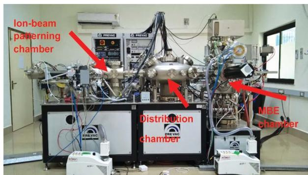
integrated with molecular beam epitaxy system for fabrication of self-organized patterned substrates, *in-situ* ultrathin films and self-assembled nanostructures to achieve nanoscale functionalities, viz. plasmonics, magnetism and optical properties. This facility is having structural characterization module and we are in the process of adding the *in-situ* compositional module as well which will make it a unique system in the country.
