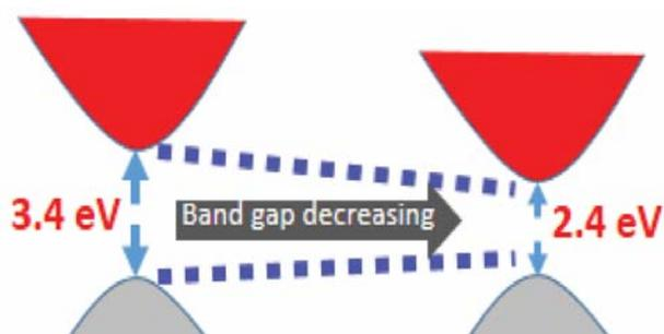
**Figure:** A schematic representation for band gap decrease in Pb doped  $\text{SnO}_2$  microstructure.
