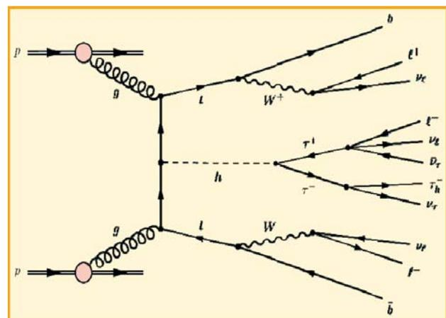
**Fig. 1:** A typical Feynman diagram for  $t\bar{t}(b\bar{b})H$  production with subsequent decay of the Higgs boson to a pair of tau leptons.
