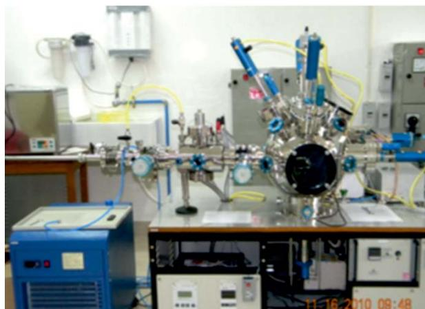
dedicated to operate with pulsed DC supply and the other two are connected to RF power supply. The substrate is made to rotate during film deposition towards having high-quality uniform films. One can put the substrate holder at a high temperature (up to 6000 C) for film growth at elevated temperatures. We have an additional and dedicated gun for deposition of three-dimensional nanostructures by using glancing angle deposition. Further, we have a load lock
