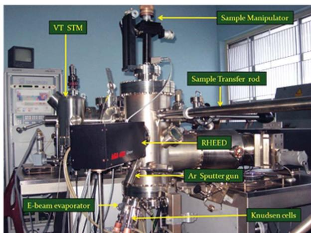
pressures (ultra high vacuum, UHV conditions) and appropriate cleaning of surfaces. The Molecular Beam Epitaxy (MBE) – Variable Temperature Scanning Tunneling Microscope (VTSTM) system is a custom designed unit procured from M/S Omicron GmbH, Germany. The facility consists of three Knudsen cells, one
