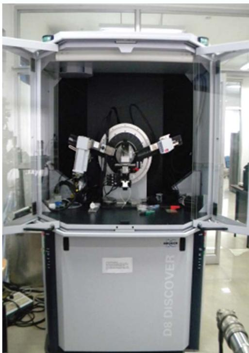
quantitative phase identification, crystal structure identification of different samples, X-ray reflectivities crystallite size determination, strain analysis and preferred orientation for established structures. In addition, we have another XRD Setup (D8, Advance), which is also in operation.
