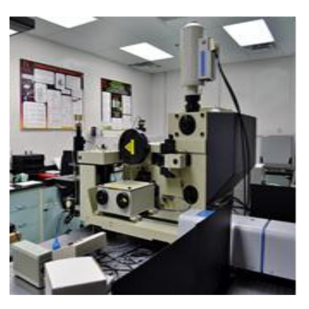
It relies on inelastic scattering of monochromatic light usually from LASER. The theory has been developed by Adolf Smeakel in 1923.
