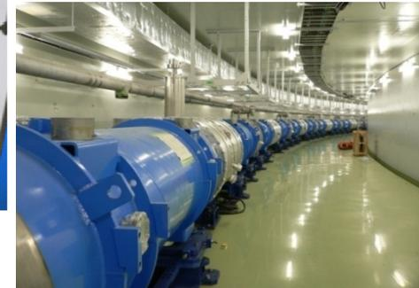
Super-conducting combined-function magnets
