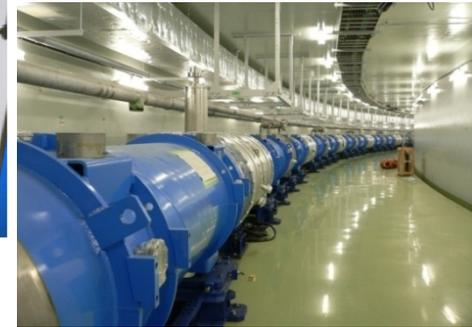
Super-conducting combined-function magnets
